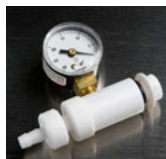
Vacuum Gauge and Bleed Valve
